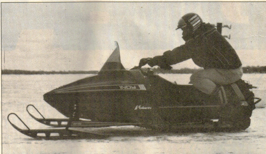
Our Indy was very, very fast out of the hole, but lost speed on top end when the hyfax overheated.
